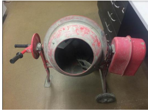
Figure 3.4: 1.25 Cubic Foot Concrete Mixer
