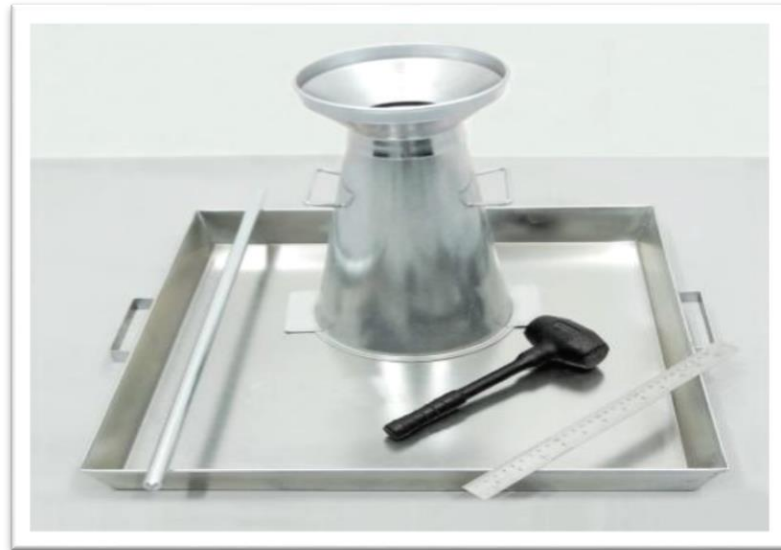
Figure 3.5 Material Set for Slump Test [6]
