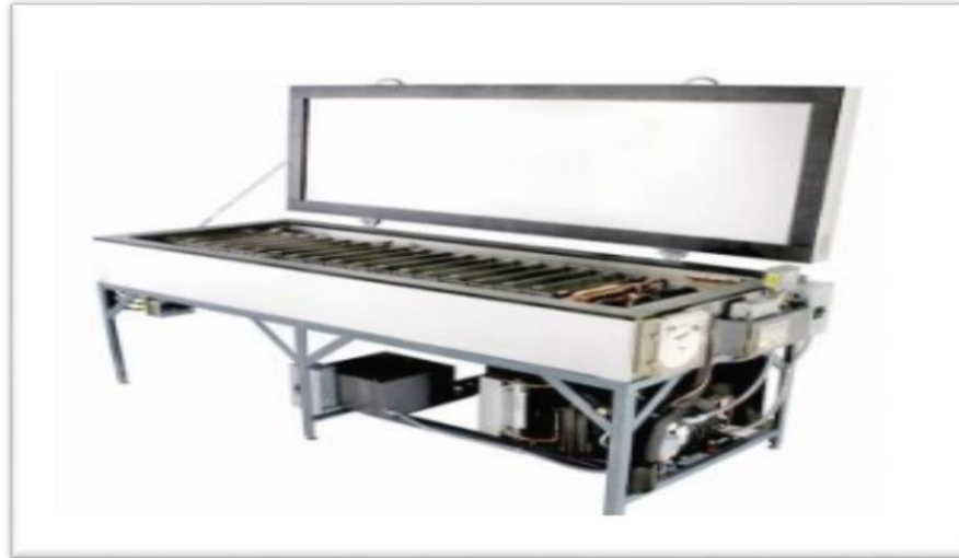
Figure 3.8: Gilson HM-120 Automatic Freeze Thaw Apparatus [7]
